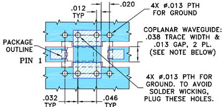
NOTE: 1. TRACE WIDTH IS SHOWN FOR ROGERS RO4350B WITH DIELECTRIC THICKNESS .020" ± .0015". COPPER: 1/2 OZ. EACH SIDE. FOR OTHER MATERIALS TRACE WIDTH MAY NEED TO BE MODIFIED.
