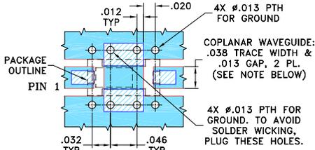
NOTE: 1. TRACE WIDTH IS SHOWN FOR ROGERS RO4350B WITH DIELECTRIC THICKNESS .020" ± .0015". COPPER: 1/2 OZ. EACH SIDE. FOR OTHER MATERIALS TRACE WIDTH MAY NEED TO BE MODIFIED.
