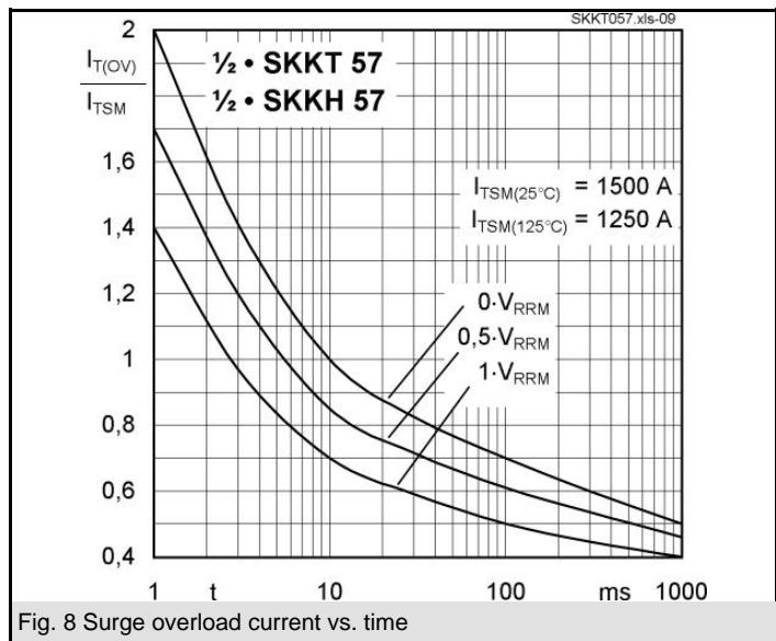
Fig. 8 Surge overload current vs. time
