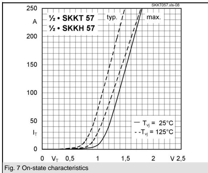
Fig. 7 On-state characteristics
