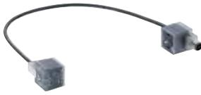
Double solenoid valve adapter (valve adapter with integrated M12 male receptacle connector), according to DIN EN 175301-803, form A, with LED function indicator and varistor for voltage protection, connected protective earth
