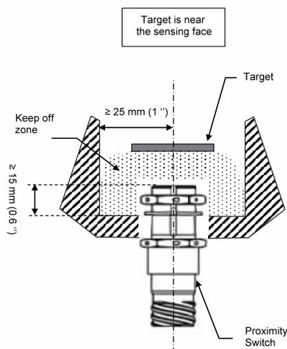
Figure 3 Keep off zone for embeddable switches
