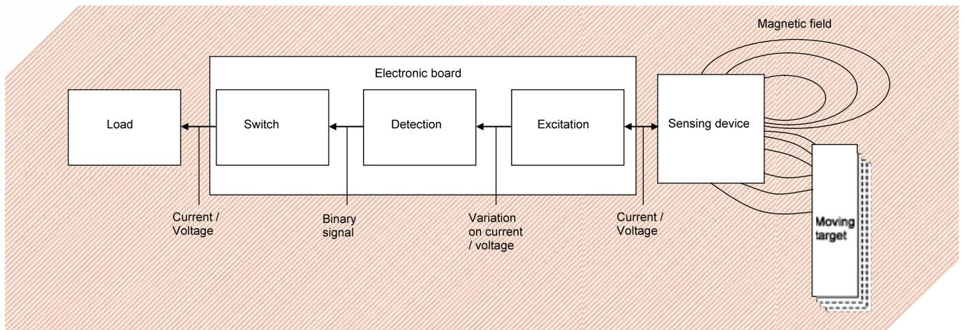
Figure 1 Measurement chain
