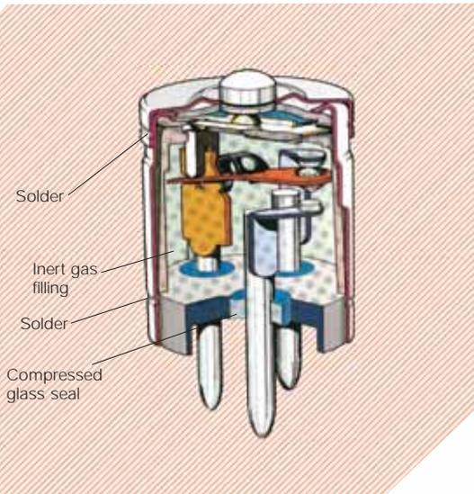
This is the basic component for our whole range of standard 1-pole and 2-poles hermetically-sealed limit switches plus the 3-poles version (special Limit Switches).
