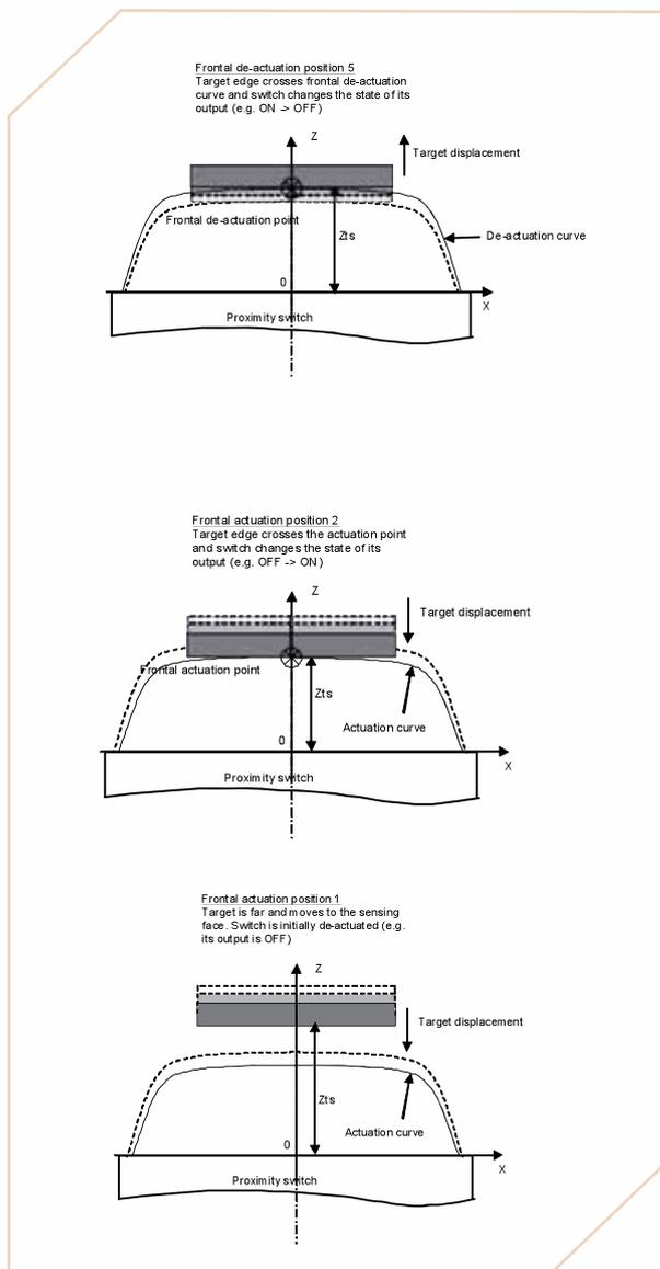
Figure 3 Target head-on actuation – deactuation point
