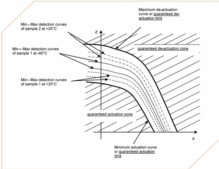
Figure 5 Definition of guaranteed detection curve and zones
