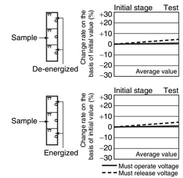
\*1. The test was conducted at an ambient temperature of 23°C.
