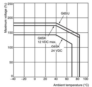
Note: "Maximum voltage" is the maximum voltage that can be applied to the Relay coil.
