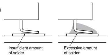
Visually check that the Relay is properly soldered.
