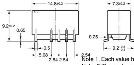
Note 1. Each value has a tolerance of  $\pm 0.3$  mm.
