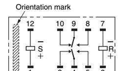
Note: Check carefully the coil polarity of the Relay.
