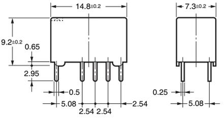
Note: Each value has a tolerance of  $\pm 0.3$  mm.
