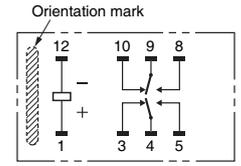
Note: Check carefully the coil polarity of the Relay.
