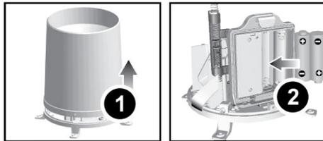
1. Remove screws and slide the cover off in an upwards motion.
