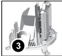
3. Remove the fibre tape.
