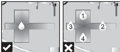
Water will pool to the center of the cross when the rain gauge is level.
