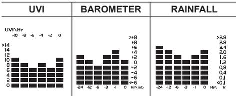
The bar chart display shows the current and historical data for the UV index, barometric pressure and rainfall readings.
