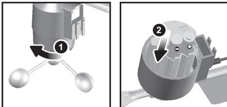
1. Unscrew the anemometer from the wind sensor carefully.
