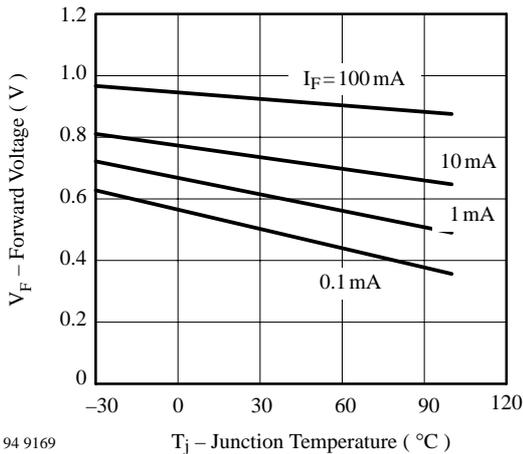
Figure 1. Forward Voltage vs. Junction Temperature
