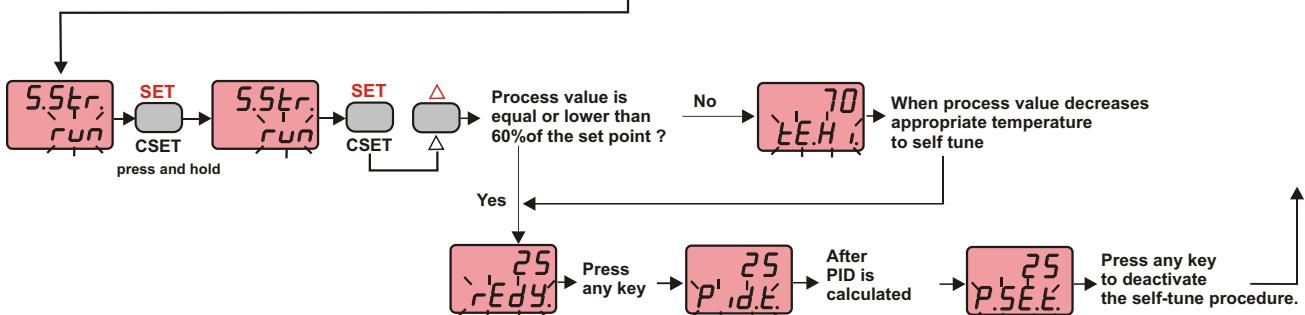
While holding **SET** key, *rUn* message flashes. Then when **CSET** key is pressed, self tune mode is entered if there is no probe failure. If process value is appropriate to begin self tune, *rEdY* message flashes. Then press any key to see *P\_id.E* message and self tune procedure begins.
