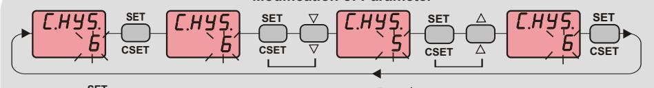
When holding **SET** key, the value of parameter flashes and using keys the requested value can be adjusted.
