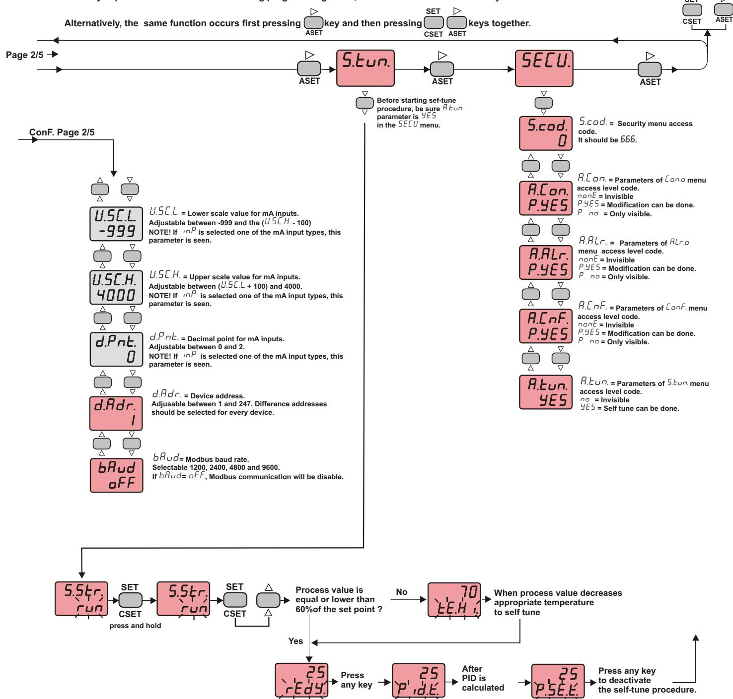
While holding **SET** key, **run** message flashes. Then when **CSET** key is pressed, self tune mode is entered if there is no probe failure. If process value is appropriate to begin self tune, **rEdy** message flashes. Then press any key to see **P.id.E.** message and self tune procedure begins.
