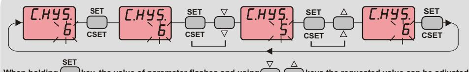
When holding **SET** key, the value of parameter flashes and using keys the requested value can be adjusted.
