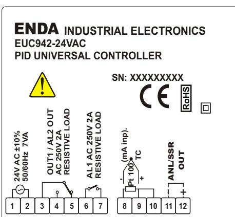
**!** Logic output of the instrument is not electrically insulated from the internal circuits. Therefore, when using a grounding thermocouple, do not connect the logic output terminals to the ground.
