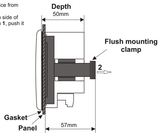
Note: 1) Panel thickness should be maximum 10mm.
