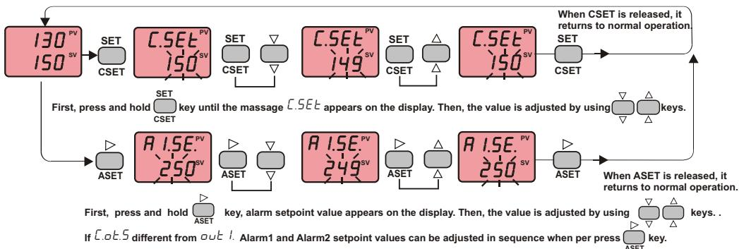
**NOTE:** The maximum of **C.SET** is the value of **C.H.L** parameter and the minimum of it is the value of **C.loL** parameter.
