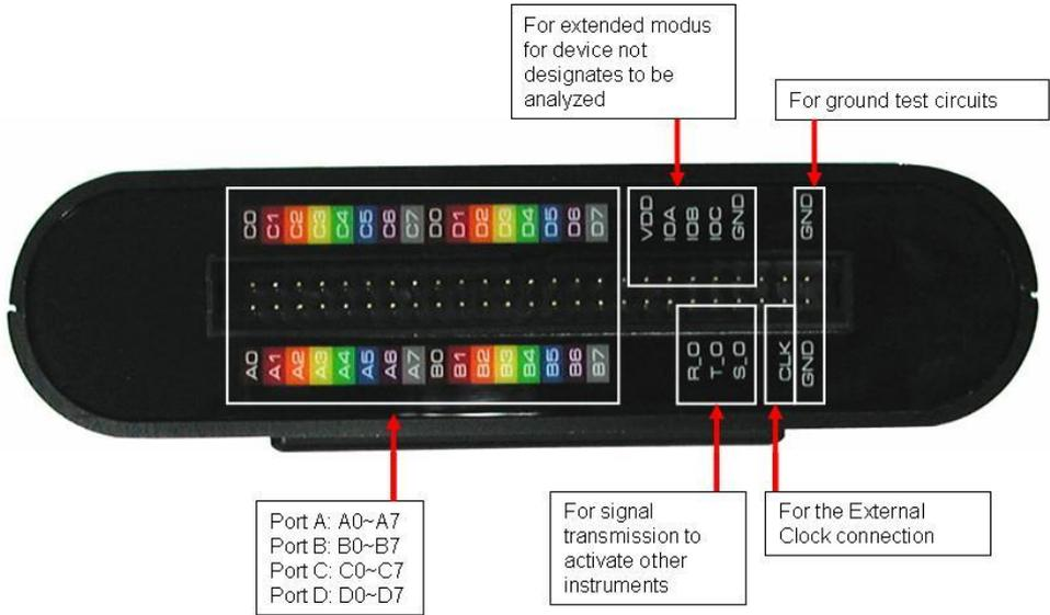
Fig. 1-11: Rear view of the Logic Analyzer ODM-A Series.
