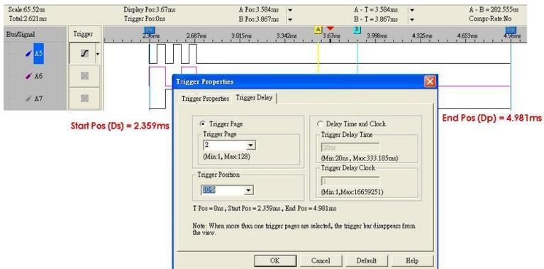
**Fig 3-11 – Trigger Position and screen**
