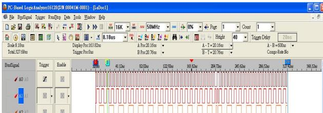
**Fig 3-13 – Trigger Position 0%**
