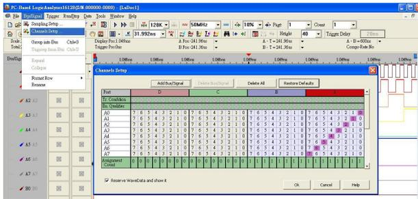
**Fig 3-21 – Channel setup**
