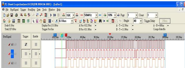
**Fig 3-14 – Trigger Position 10%**
