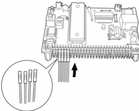
2. Plug the loose ends into the connectors on the circuit board to be analyzed (Fig.2-2).
