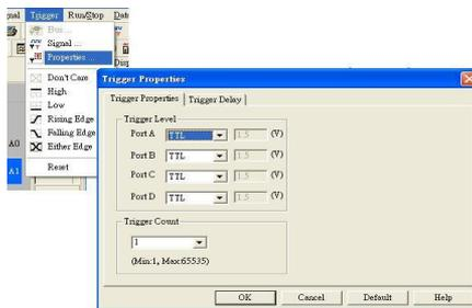
**Fig 2-4 – Trigger Properties**
