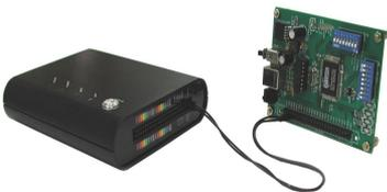
3. The circuit board must be grounded to the Logic Analyzer with the connecting cables (Fig.2-3).
