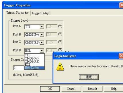
Fig 2-5 – Trigger Properties Error
