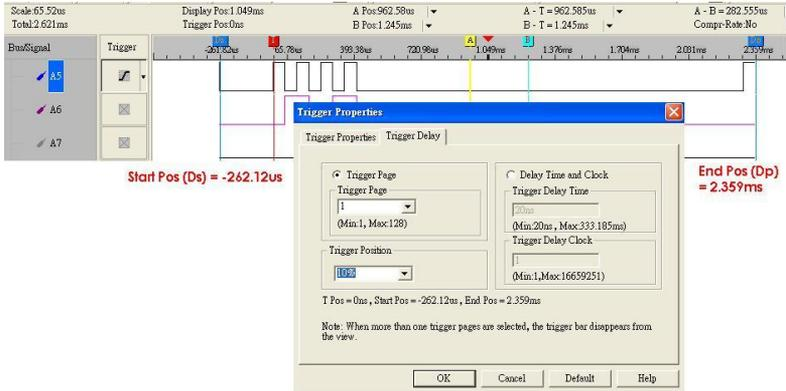
**Fig 3-10 – Trigger Position**
