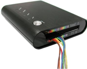
1. Plug the fixed end of the cables into the LA (Fig.2-1).
