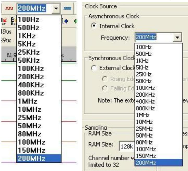
**Fig 2-2 – Clock source drop down menu**
