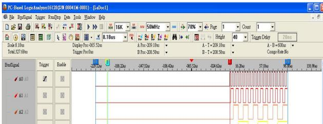
**Fig 3-15 – Trigger Position 70%**
