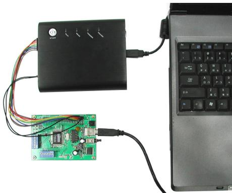
Fig. 2-6: An assembly of Laptop, Logic Analyzer, and a testing board.
