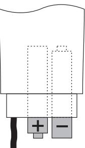
The batteries need to be changed when the yellow indicator (E) no longer lights up when the two test tips (1 and 11) contact each other, and no signal tone sounds.
