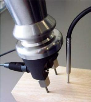
**Reciprocating piston electrode GHE91 with temperature-probe GTF38**
