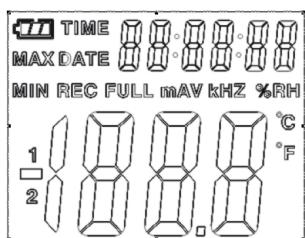
1. This battery sign will be displayed if battery is fully charged. When battery is exhausted, sign will be displayed. At that time, replacing a new battery is necessary.
